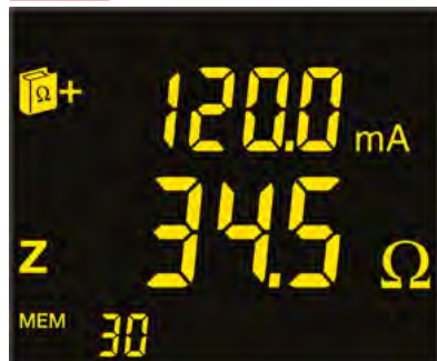
Screen 1: Impedance and leakage current
