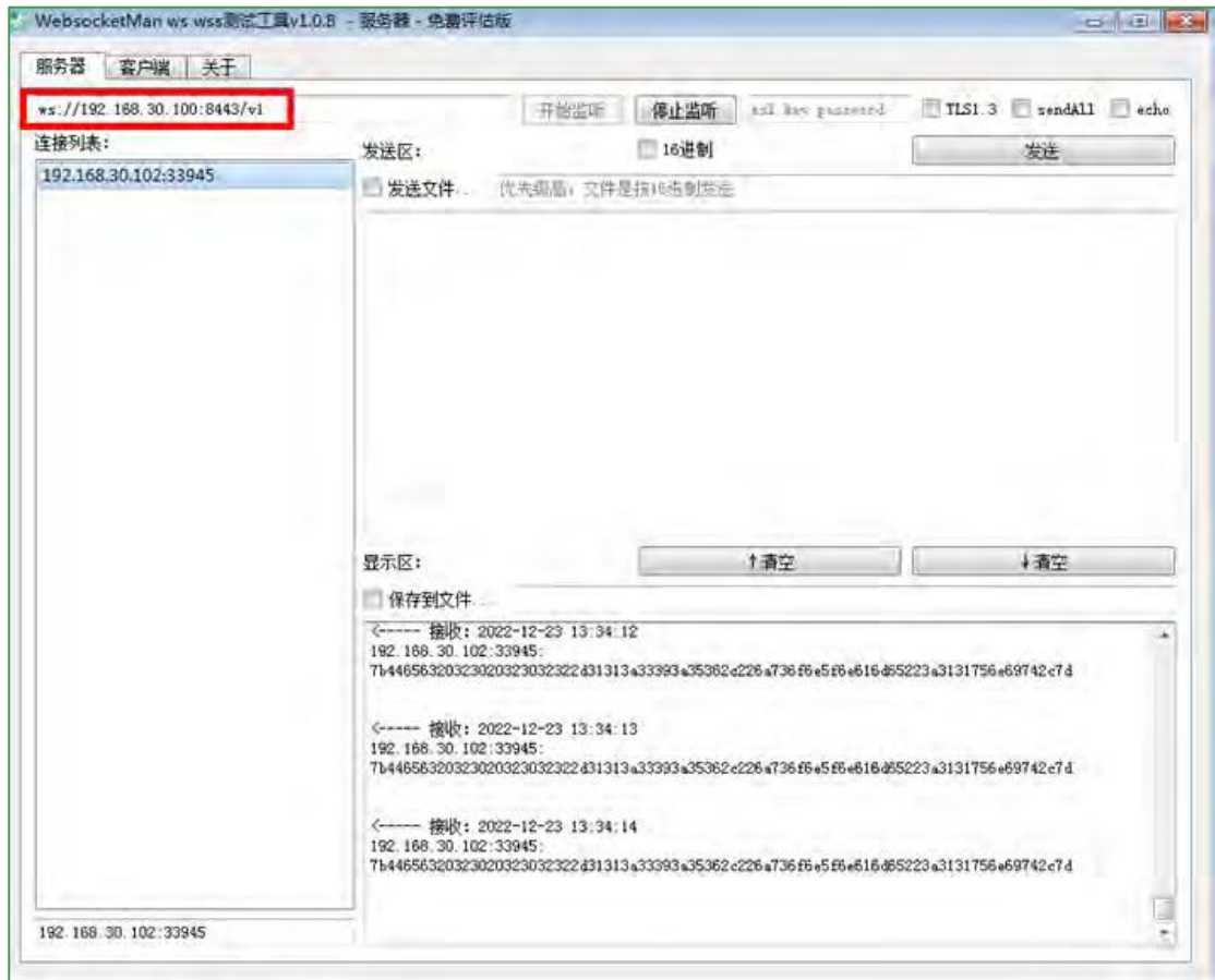
Figure 4-35 Websocket server configuration example
