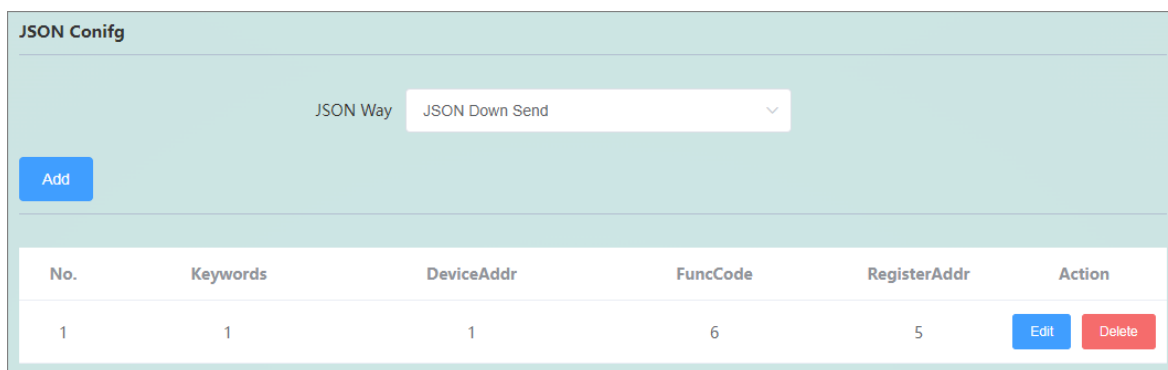
Figure 4-38 Configuration example of sending JSON parameters
