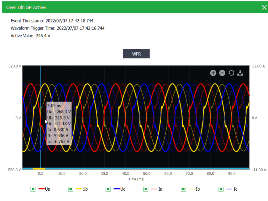
Figure 3-108 Over Uln Setpoint Active
