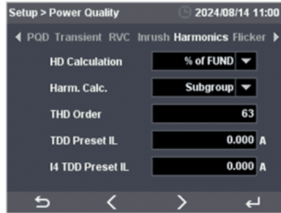
Figure 4-11 PQ-Harmonics Setup Interface
