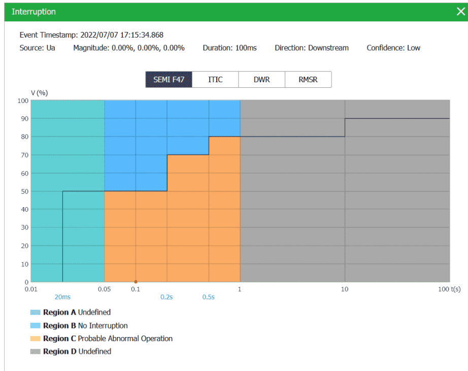
Figure 3-109 Interruption on SEMI F47 Interface
