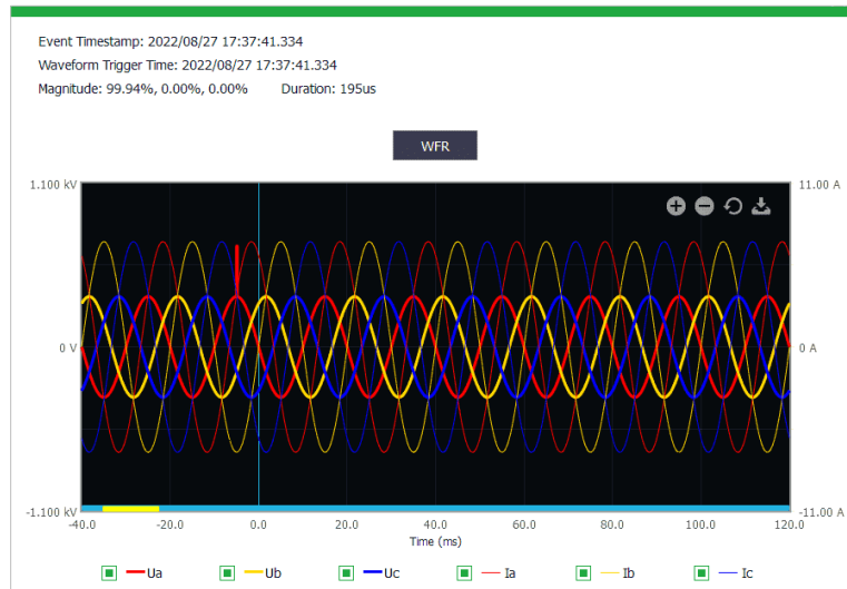
Figure 4-9 Transient Event @ 512 samples/cycle x 100 cycles
