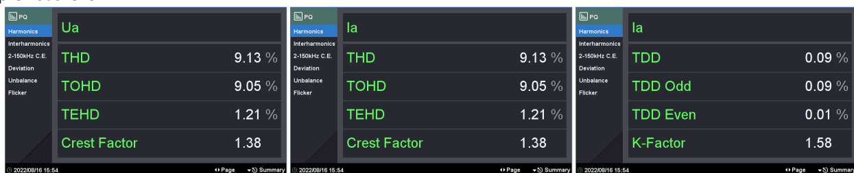
Figure 3-21 Voltage and Current Harmonics Large Font Displays
