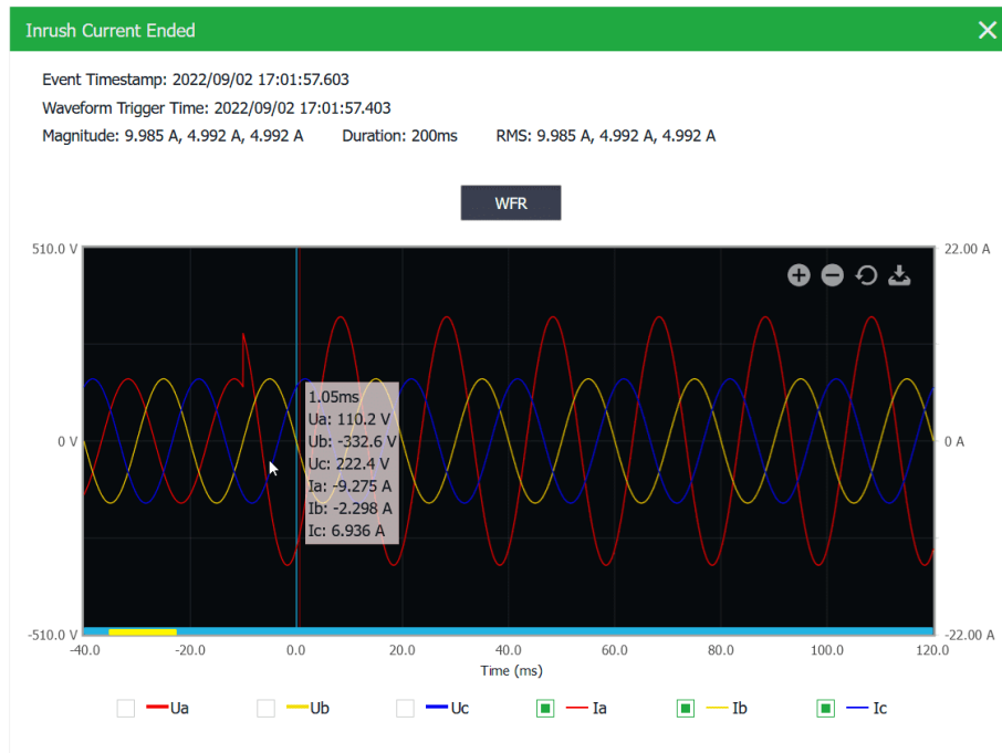
Figure 4-17 Inrush Current - displayed on Web Server
