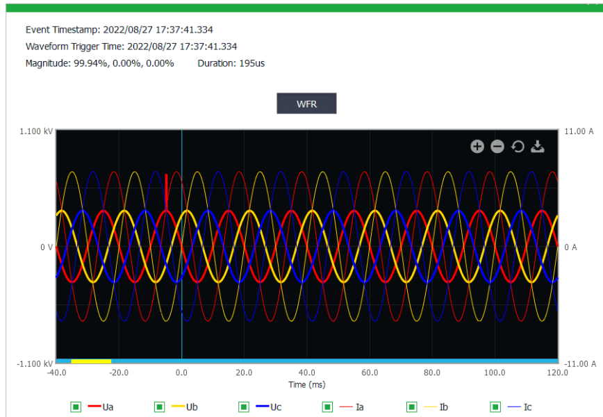
Figure 4-9 Transient Event @ 512 samples/cycle x 100 cycles
