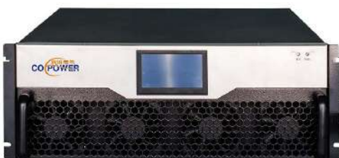
▲ 75A Rack-Mounted APF – 35kg 550.6W x 540D x 190H (mm)
